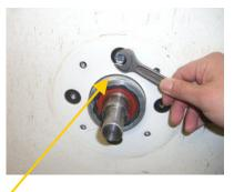
Lean the wheel upside down and support it so that the shaft does not touch the ground. Take off the last bolt by supporting motor from the other side
