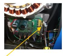
Unscrew the cable holder and cut the the zip tie to release the cables for the motor
