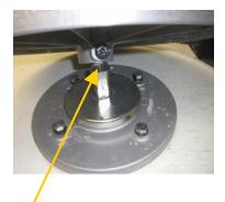
The wheel head bolt must be tightened onto the flat part of the shaft. If it is not on properly, the shaft will spin but the wheel head will not have any torque.
