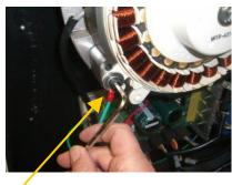
Remove the green ground wire found attached to the motor
