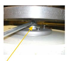
Use the T-wrench to loosen the screw to remove the wheel head
