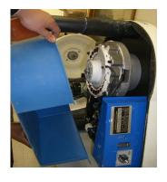
Place the wheel vertical and remove the undercover by removing all undercover screws then sliding the undercover off.
