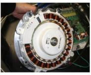
Once the motor is completely detached, lift it out and replace it with the new motor.
