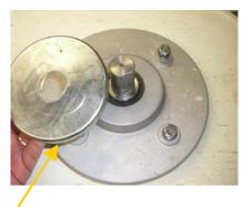
Remove the metal cover from the shaft that fits over the bearing plate
