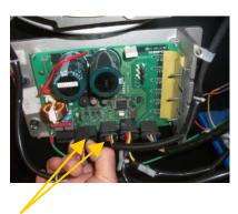
Un-clip the 2 connections from the control board for the motor by squeezing the sides of the clip and pulling.
