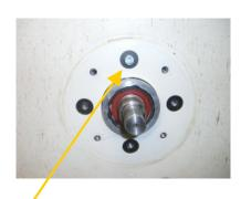
Place the first bolt back in and tighten. Then lean the wheel to a vertical position again. Replace all parts in the same way they were taken off.
